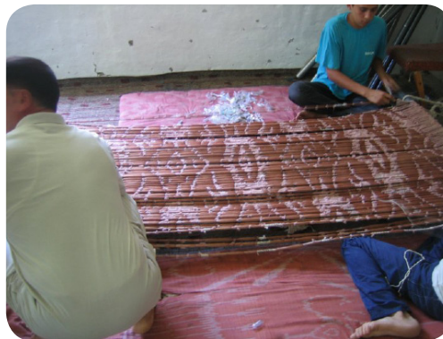
A warp stretched for its second round of resist bindings. It has been dyed and the first layer of resists must be taken off so that another layer can be put on.
