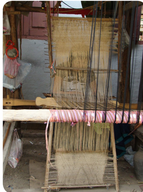
The design of the template-pattern can be clearly seen on this loom. After each horizontal memory-thread, which represents a line of pattern in the weft, is used, it is moved from the template's top to the bottom; later, the memory threads will be moved from bottom to top, creating the traditional mirror-image motifs in the design-work.
