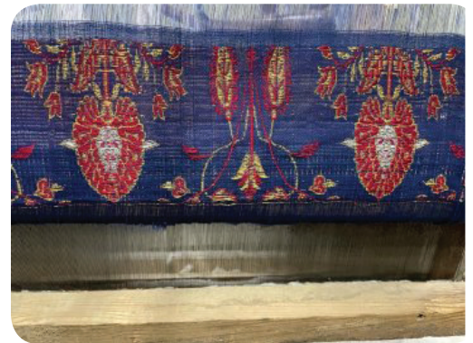
The drawloom technique enables designs to have a much larger scale than typical jacquard looms and hence the Ramzani Jangla has a stunning tapestry like effect
