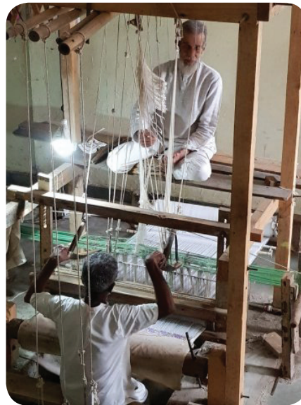
The Paaga Loom or drawloom is operated by two people--the weaver and the “draw-boy” who lifts the warp threads
